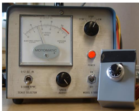
Figure 4. Motor Speed Control; use the knob on the small attached box, not on the motor.
