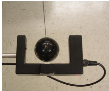
Figure 1. (a) Pendulum support stand with metal and wood bobs resting on the table, optical gate, and calipers. (b) The pendulum bob hangs from a string held by an upper support clamp and a lower support arm. (c) Pendulum string passing through photogate timer as it oscillates with a small amplitude.
